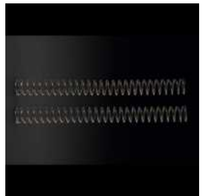
FRONT FORK SPRING K=2.75 N/MM £27.35
