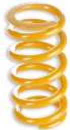
Rear shock absorber spring K=105 N/mm £205.94
